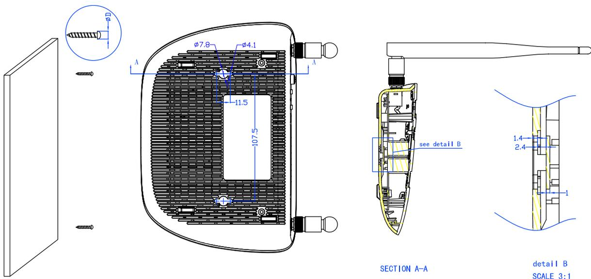
Figure 2-1 Wall-mount Install
