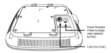
\* PoE kit (injector and adapter) is NOT include in the package and it can be purchased with the model name "DPE-301GI".
