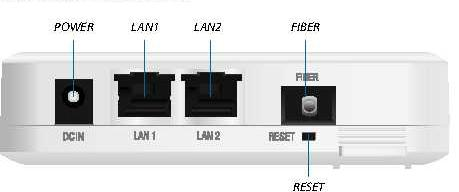
**DCIN** The Power Adapter is connected here.
