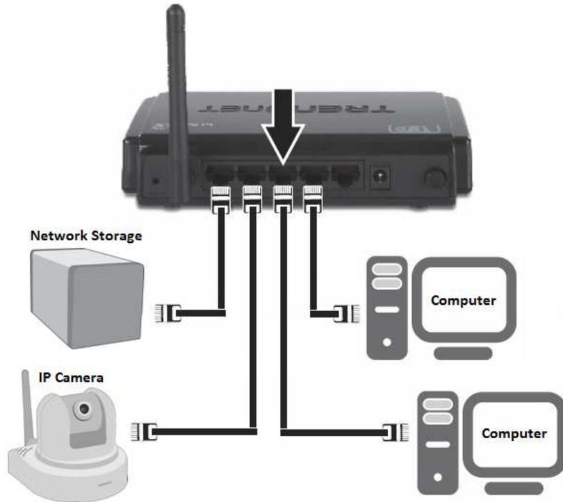
The router is installed near the modem (typically supplied by your ISP "Internet Service Provider") and physically connected to it from the router's WAN port to the modem's network port which connects to the Internet. Wireless signals from the router are broadcasted to wireless clients such as laptops (with wireless capability) thereby providing Internet access.
