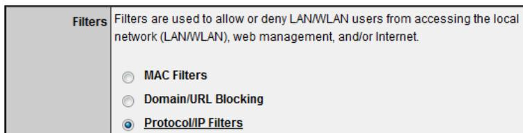
To simplify configuration, there is a list of commonly used pre-defined Protocol/IP Filters to modify otherwise, you can choose to manually add a new Protocol/IP Filter.
