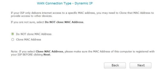
Figure 3-6 Quick Setup - MAC Clone
