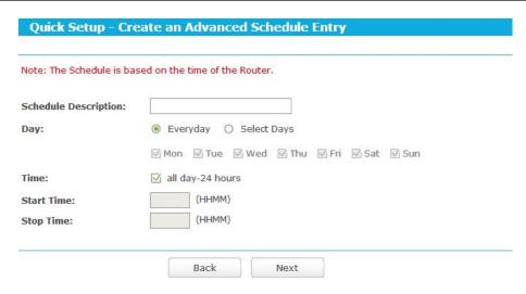
Figure 5-63 Quick Setup – Create an Advanced Schedule Entry
