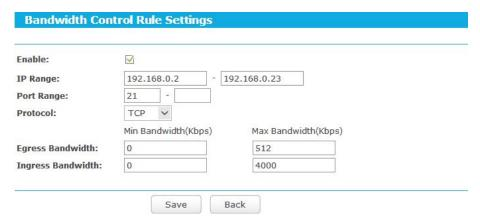
Figure 5-79 Bandwidth Control Rule Settings
