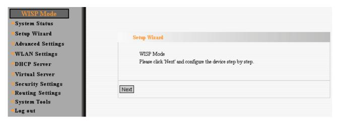
In WISP mode, ZSR4174WE will behave just the same as the Client mode for wireless function. However, router functions are added between the Wireless WAN side and the Ethernet LAN side. Therefore, the WISP subscriber can share the WISP connection without the need for extra router. The NAT is enabled and PCs in Ethernet ports share the same IP address assigned by DHCP function to ISP through wireless LAN.
