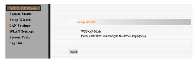
In WDS+AP mode, ZSR4174WE will work similar as WDS mode. It supports the wireless bridge between the two wired networks; the connection of wireless network is also supported at the same time.
