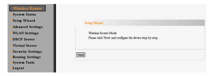
In Wireless Router mode, ZSR4174WE will behave as the router with wireless NAT function and DHCP sever. And PCs can get the IP address automatically assigned by DHCP server.
