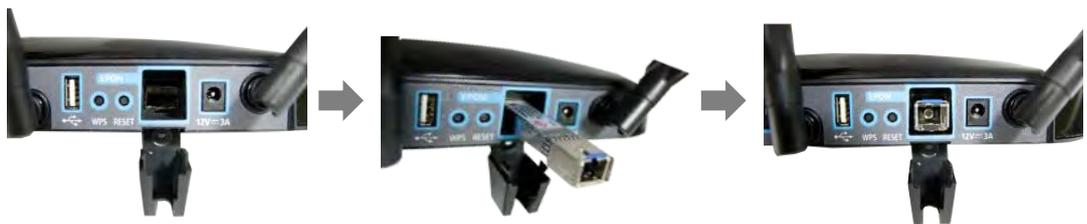
Step 3: Connect the SC/APC connector on one end of a single-mode optical fiber into the optical terminal of the optical outlet (it could be a splitter or PIM card of an OLT) and the other end into the PON port of C1004W by pushing it until a click sound is heard.
