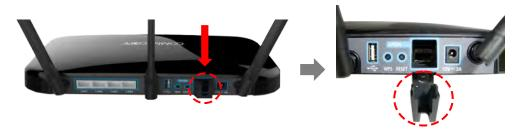
**Step 2:** Slide the 10G SFP+ optic module into the socket on the ONU.
