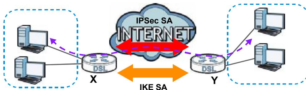
In this example, a computer in network A is exchanging data with a computer in network B. Inside networks A and B, the data is transmitted the same way data is normally transmitted in the networks. Between routers X and Y, the data is protected by tunneling, encryption, authentication, and other security features of the IPsec SA. The IPsec SA is established securely using the IKE SA that routers X and Y established first.
