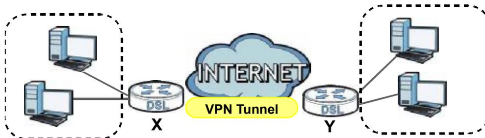
The VPN tunnel connects the NBG5715 (X) and the remote IPSec router (Y). These routers then connect the local network (A) and remote network (B).
