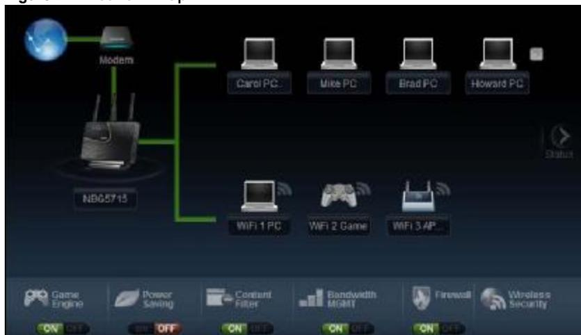
The line connecting the NBG5715 to the gateway becomes green when the NBG5715 is able to ping the gateway. It becomes red when the ping initiating from the NBG5715 does not get a response from the gateway. The same rule applies to the line connecting the gateway to the Internet.
