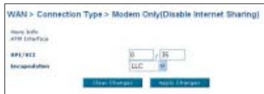
1. **VPI/VCI** - Enter your Virtual Path Identifier (VPI) and Virtual Circuit Identifier (VCI) parameter here. (Assigned by your ISP).
