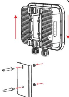
(2) Screw the anchors into the holes until they are flush with the wall.
