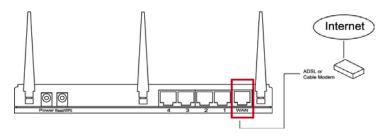
2. Connect all your computers, network devices (network-enabled consumer devices other than computers, like game console, or switch / hub) to the LAN port of the router.
