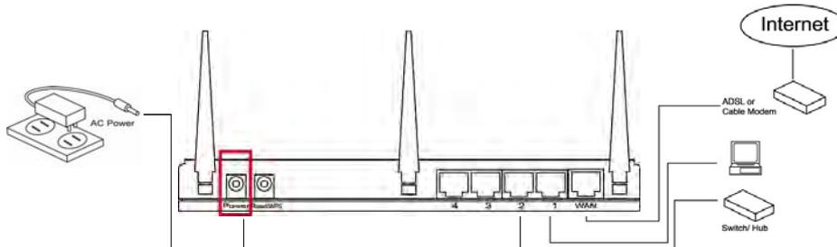
4. Please check all LEDs on the front panel. 'PWR' LED should be steadily on, WAN and LAN LEDs should be on if the computer /
