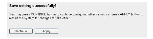
Press 'Continue' to save the settings made and back to web management interface; press 'Apply' to save the settings made and restart the router so the settings will take effect after it reboots.
