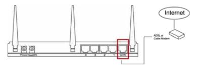
2. Connect all your computers, network devices (network-enabled consumer devices other than computers, like game console, or switch / hub) to the LAN port of the router. If you are connecting to Gigabit network, please use Cat. 5e cable at least.
