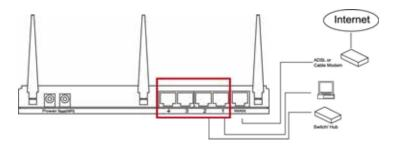
3. Connect the A/C power adapter to the wall socket, and then connect it to the 'Power' socket of the router.
