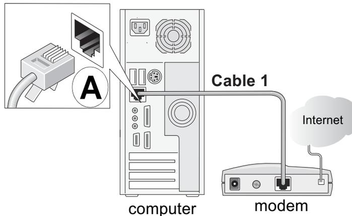
**Figure 3-2: Disconnect the Ethernet cable from the computer**
