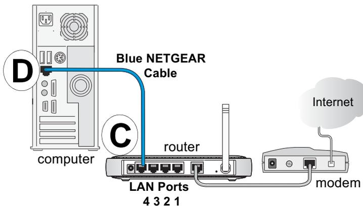
**Figure 3-4: Connect the computer to the wireless router**
