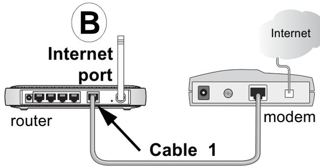
**Figure 3-3: Connect the wireless router to the modem**
