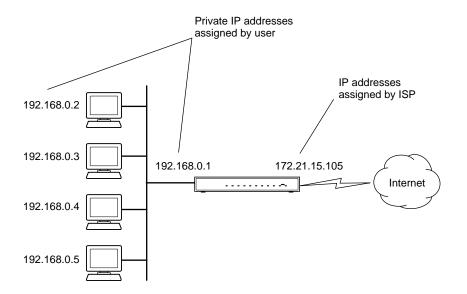
The following figure illustrates a single IP address operation.
