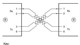
B = Normal or MDI-X port (as on a hub or switch) 1, 2, 3, 6 = Pin numbers
