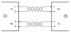
Key: A = UPLINK OR MDI PORT (as on a PC) B = Normal or MDI-X port (as on a hub or switch) 1, 2, 3, 6 = Pin numbers
