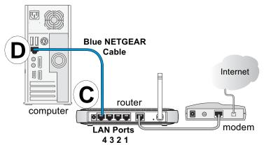
Figure 3-4: Connect the computer to the wireless router
