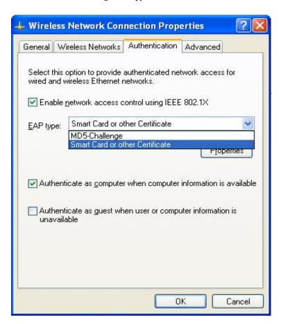
Figure 2: Enable IEEE 802.1X access control
