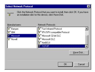
6. The TCP/IP protocol shall be listed in the Network window. Click **OK** to complete the install procedure and restart your PC to enable the TCP/IP protocol.
