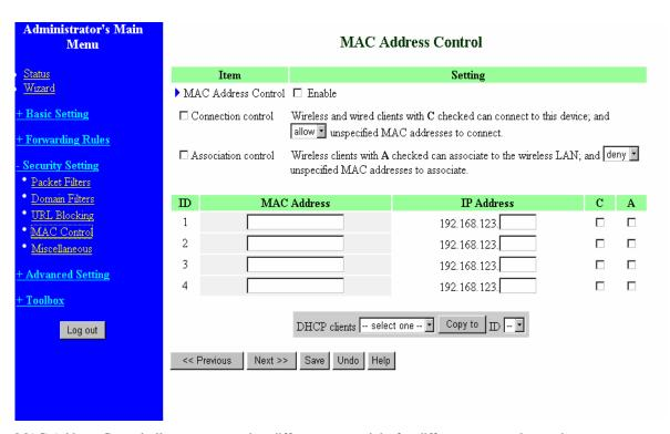
MAC Address Control allows you to assign different access right for different users and to assign a specific IP address to a certain MAC address.
