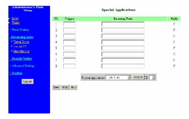
Some applications require multiple connections, like Internet games, Video conferencing, Internet telephony, etc. Because of the firewall function, these applications cannot work with a pure NAT router. The **Special Applications** feature allows some of these applications to work with this product. If the mechanism of Special Applications fails to make an application work, try setting your computer as the **DMZ** host instead.
