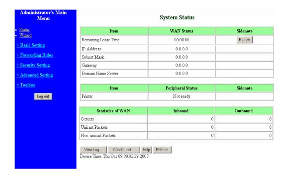
Activate your browser, and **disable the proxy** or **add the IP address of this product into the exceptions**. Then, type this product's IP address in the Location (for Netscape) or Address (for IE) field and press ENTER. For example: <a href="http://192.168.123.254">http://192.168.123.254</a>.
