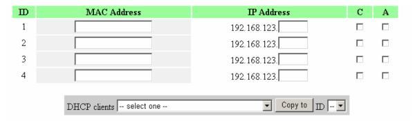
"Control table" is the table at the bottom of the "MAC Address Control" page. Each row of this table indicates the MAC address and the expected IP address mapping of a client. There are four columns in this table:
