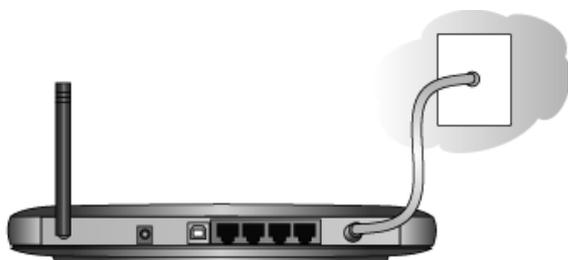
**Figure 3-1: Connect the gateway to the cable network.**
