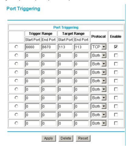
Figure 5-7: Port Triggering menu, with IRC example.
