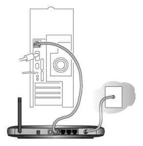
Figure 3-2: Connect a PC to the gateway
