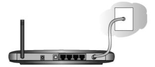
Figure 3-1: Connect the gateway to the cable network.
