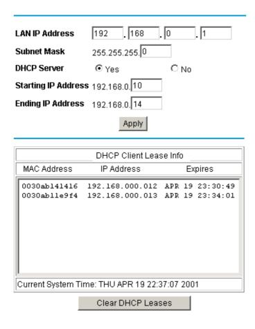
Figure 6-3: LAN IP setup screen.
