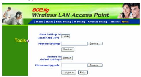
Save Settings to Local Hard Drive: Click on "Save Settings to Local Hard Drive" button, which will open a FileSave Dialog box, where user gets to save all the current settings and configurations to a file.
