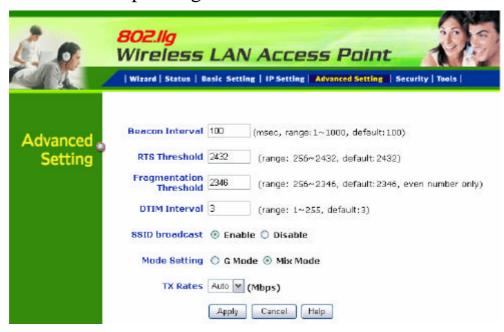
**Beacon Interval:** To set the period of time in milliseconds that AP sends out a beacon. Default is 100 milliseconds.
