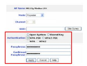
**Apply:** For the changes made to any of the items above to be effective, click "Apply". The new settings are now been saved to Access Point and will be effective once the Access Point restarts.
