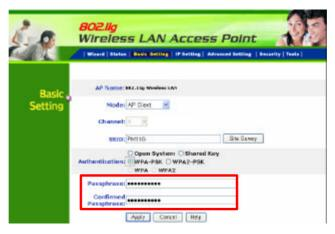
**Apply:** For the changes made to any of the items above to be effective, click "Apply". The new settings are now been saved to Access Point and will be effective once the Access Point restarts.
