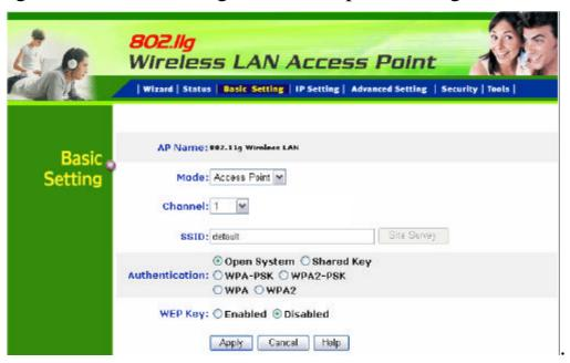
**AP Name:** The name of the AP, which can be used to identify the Access Point among the all the Access Points in the wireless network.
