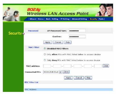
**Password**: Allow user to change the new login password. Here are the necessary steps:
