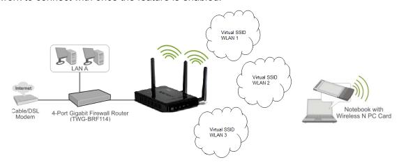
Multiple SSID (Virtual WLANs)
