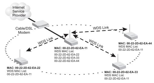
Figure 46: Manual WDS MAC Address Configuration
