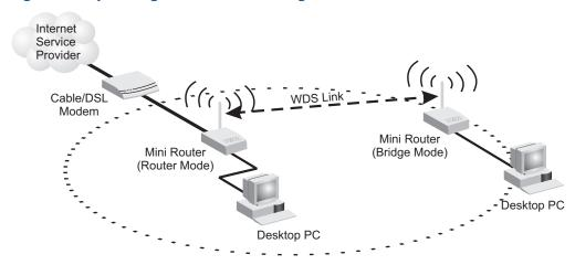
Figure 8: Operating as a Wireless Repeater
