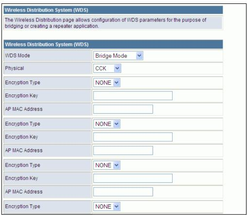
The WDS settings configure WDS related parameters. Up to four MAC addresses can be specified for each unit in the WDS network. WDS links may either be manually configured (Bridge and Repeater modes) or auto-discovered (Lazy mode).
