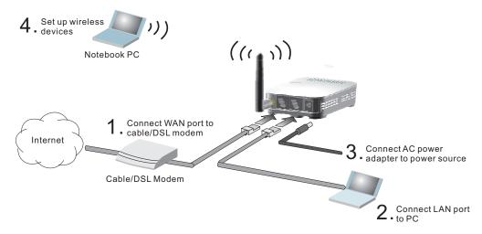
To connect the Mini Broadband Router in Router Mode for use as an Internet gateway, follow these steps:
