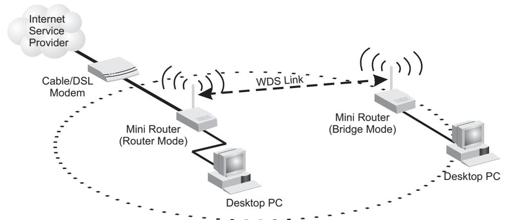
**Figure 8: Operating as a Wireless Repeater**
