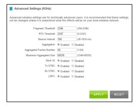
Beacon Interval: Indicates the frequency interval of the beacon. A beacon is a packet broadcast by the Range Extender to sync the wireless network.
