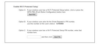
Option A: Push button: You may push the WPS button on the web menu or use the physical button on the top of the Range Extender.
