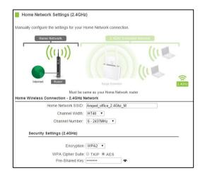
Channel Width: Wi-Fi operates in two separate channel widths, 20Hz and 40Hz. 40Hz allows for faster speeds. Each Channel Width will have a different selection of wireless channels to choose from. Select the channel
