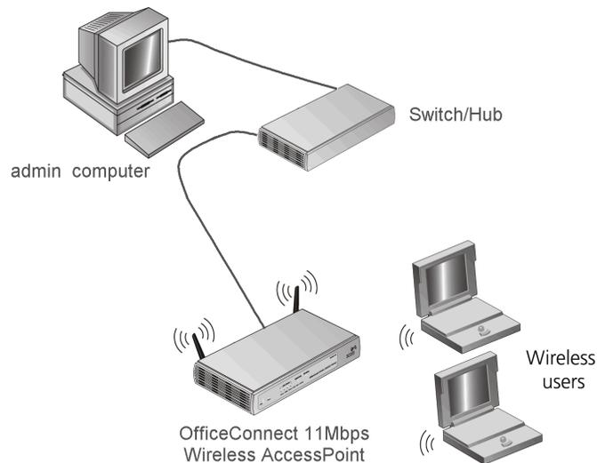
To use your Access Point to connect to the wireless LAN to the wired LAN:
