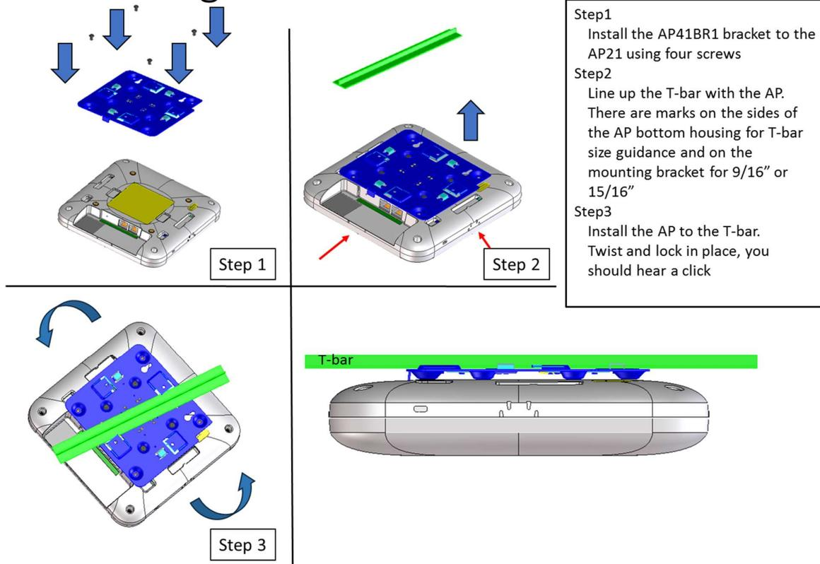
When mounting to a T-bar, please use the screws that are provided which have a head diameter of 8mm and a length of 6mm.
