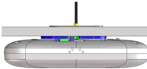
When mounting to an acoustic ceiling tile, please use the screws that are provided which have a head diameter of 7mm and a length of 40mm.
