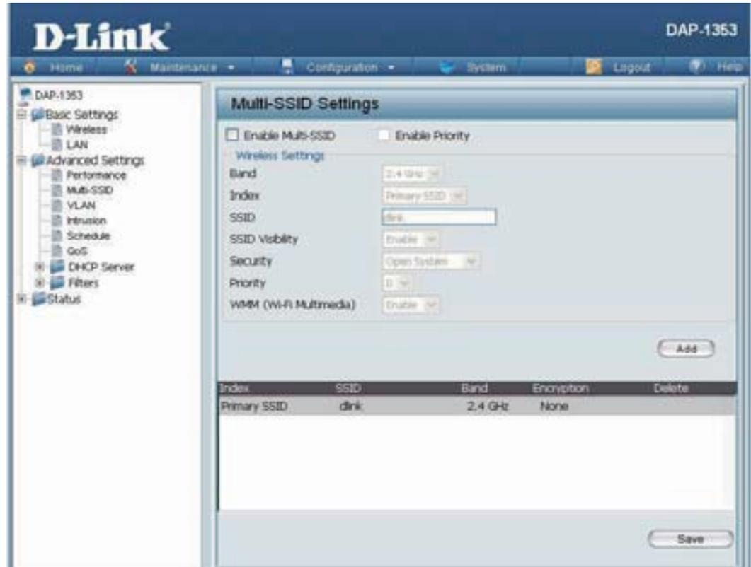
**Enable Multi-SSID:** Check to enable support for multiple SSIDs.
