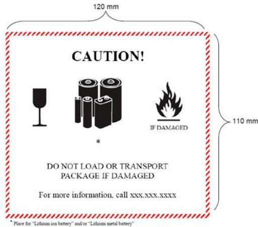
Label content for shipping smaller packages for batteries:
