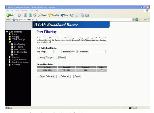
Screen snapshot – Firewall - Port Filtering
