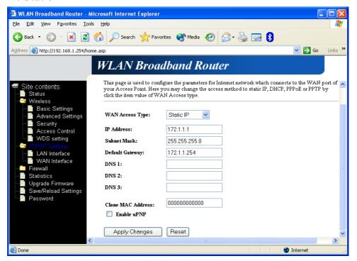
Screen snapshot – WAN Interface Setup – Static IP
