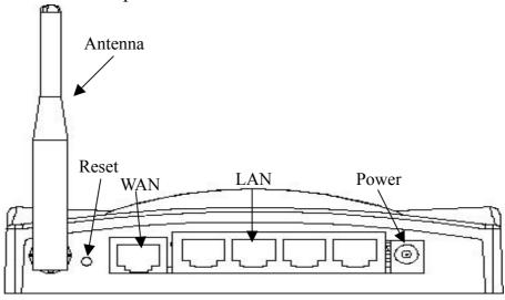
Figure 2 – WLAN Broadband Router Rear Panel
