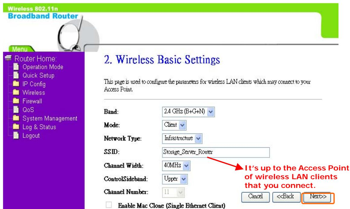
The screenshot shows the configuration page for wireless LAN clients. The page title is "2. Wireless Basic Settings". A navigation menu on the left includes: Router Home, Operation Mode, Quick Setup, IP Config, Wireless, Firewall, QoS, System Management, Log & Status, and Logout. The main content area contains the following settings:
