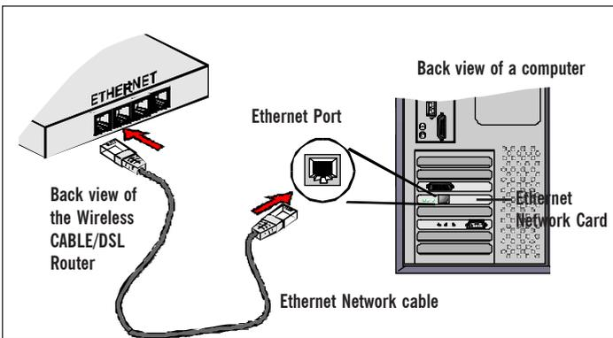
(All the Ethernet Ports on the CABLE/DSL Router are Auto MDI/MDIX. Both Straight and Cross Ethernet Network cables can be used).
