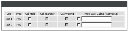
Call Hold: Check the box to hold the call on the specific FXS port.
