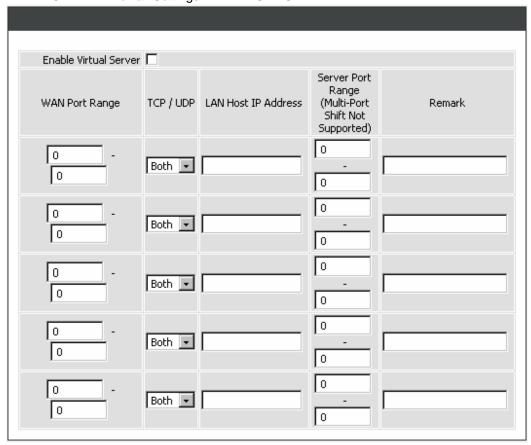
**Enable Virtual Server:** Check the box to enable port forwarding.
