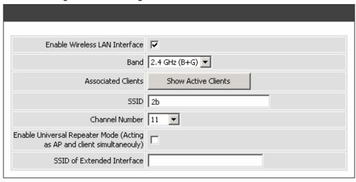
Enable Wireless LAN Interface: Enable wireless basic settings on LAN interface.
