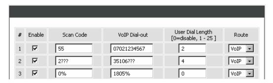
Pick up the handset and dial 0423456789. The gateway will dial 0423456789 and go through Internet first. If the call is fail to Internet, the gateway will dial 1805423456789 and go through PSTN/FXO. You also can use Digit Map Testing to see the result of what gateway will dial.
