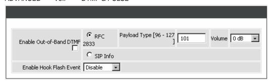
**Enable Out-of-Band DTMF:** This variable is to set the method of DTMF transmission. RFC2833 or SIP Info.
