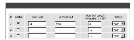
Pick up the handset and dial 11. The gateway will dial "test" and go through Internet. You also can use Digit Map Testing to see the result of what gateway will dial.
