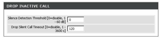
This feature is a call drop standard for a gateway to determine whether or not to hang up the phone. The gateway will disconnect the call automatically to avoid keeping the line engaged if the detected volume is below the **Silence Detection Threshold** or the time exceeds the **Drop Silent Call Timeout**.
