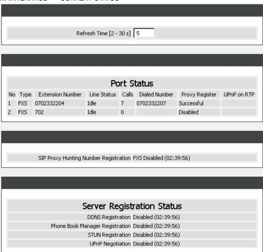
For Port Status, it includes if each port registers to Proxy successfully, the last dialed number, how many calls each port has made since the gateway is start, etc.
