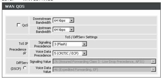
**QoS:** Check the box to guaranty the voice quality. Voice packets have the highest priority in IP networks, and the data transmission is distributed to less bandwidth.
