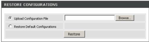
**Upload Configuration File:** Once you locate the file, click **Upload** to overwrite the current settings with the settings saved to the file.
