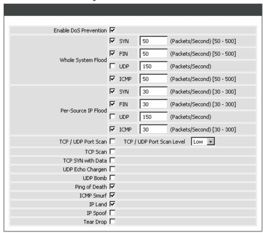
**Enable DoS Prevention:** Check the box to prevent DoS attacks from WAN or LAN. There are various types of DoS attacking. Leave settings in this field to the default if you are not familiar with it.
