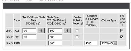
**Min. FXS Hook Flash Time:** Enter the minimum flash time for FXS detecting. When the flash signal generated by the phone set is shorter than Min. FXS Hook Flash Time, FXS port will be on-hook.
