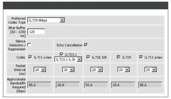
**Preferred Codec Type:** Select a preferred codec type for all calls. Since different voice codecs have different compression ratios, the sound quality and occupied bandwidths are also different. The factual codec may determine by the called party. It is recommended that you use the default provided (G.723.1) codec because it occupies less bandwidth and provides better sound quality.
