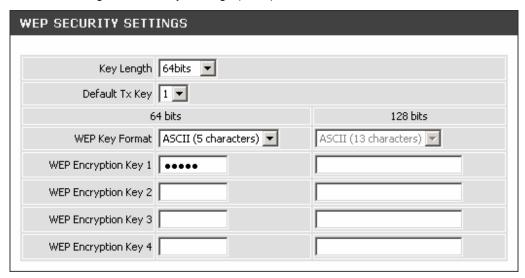
Key Length: Select 64-bit or 128-bit data encryption.
