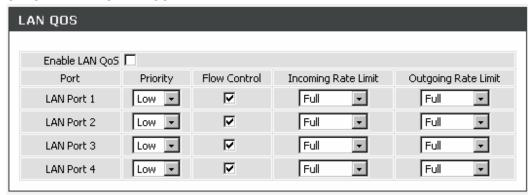
Enable LAN QoS: Check the box to enable LAN QoS by Hardware.
