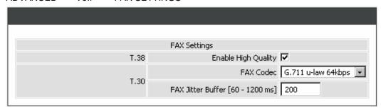
**Enable High Quality:** Check the box to increase approximately two times the bandwidth in order to compensate possible loss of packet during transmission and offers a better and reliable fax quality.
