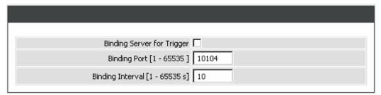
**Binding Server for Trigger:** Check the box to trigger a connection between Provisioning Server and the gateway. Provisioning Server will bind a port for the gateway to send provision request.
