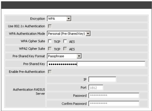
Select the type of WPA-PSK (WPA-PSK, WPA2-PSK, WPA2 Mixed-PSK), choose the proper security mode according to your wireless network.
