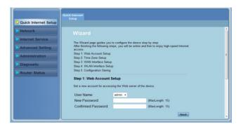
In Step 2: Time Zone Setup page, tick Enable to enable the NTP function, and key in the necessary information. Click Next.
