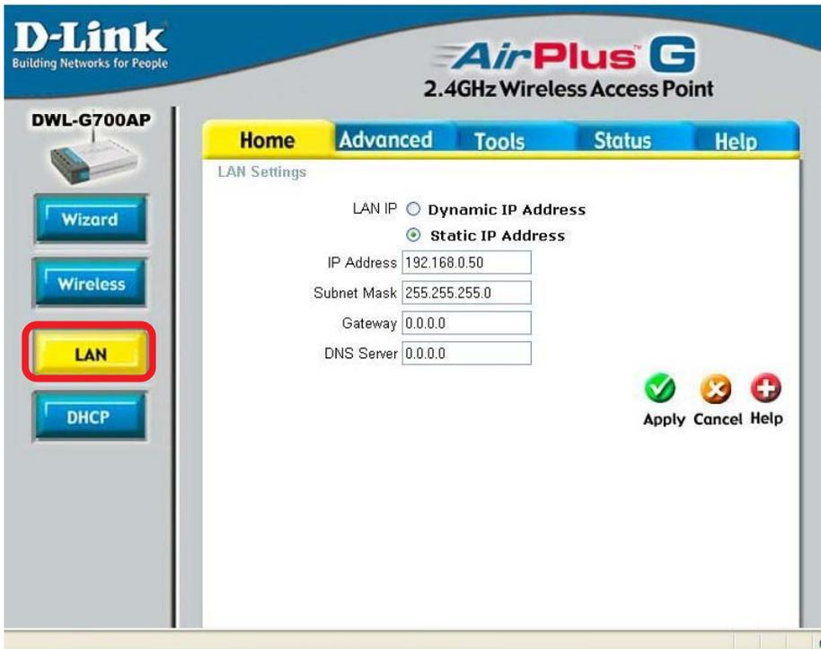
**Dynamic IP Address:** Select this option if you would like to have an IP Address automatically assigned to the DWL-G700AP by a DHCP server in your network.
