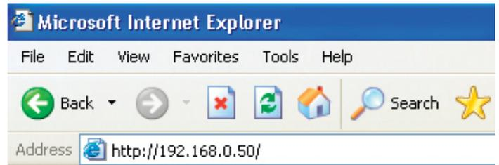
*Note: If you have changed the default IP address assigned to the DWL-G700AP, make sure to enter the correct IP address.*
