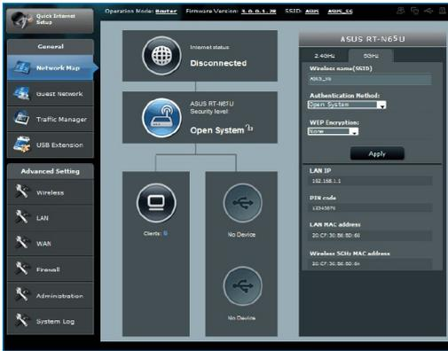
4. On the **Wireless name (SSID)** field, key in a unique name for your wireless network.
