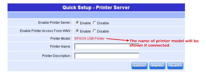
Enable the printer and the Printer Model will be shown when plug in. Please click on "**Next**" button to connect to next setup.
