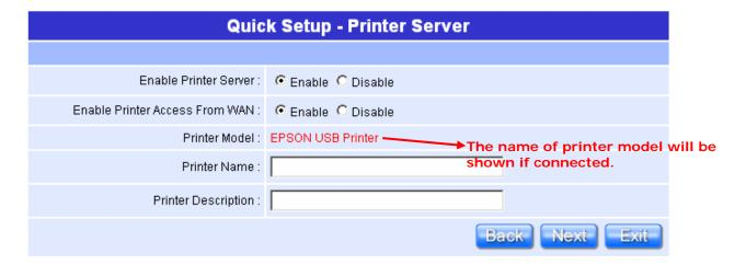
Enable the printer and the Printer Model will be shown when plug in. Please click on "**Next**" button to connect to next setup.
