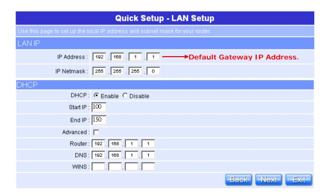
Please don't change the default LAN IP settings at this point until you have completed the rest of the configurations and confirm that your Internet connection is working.
