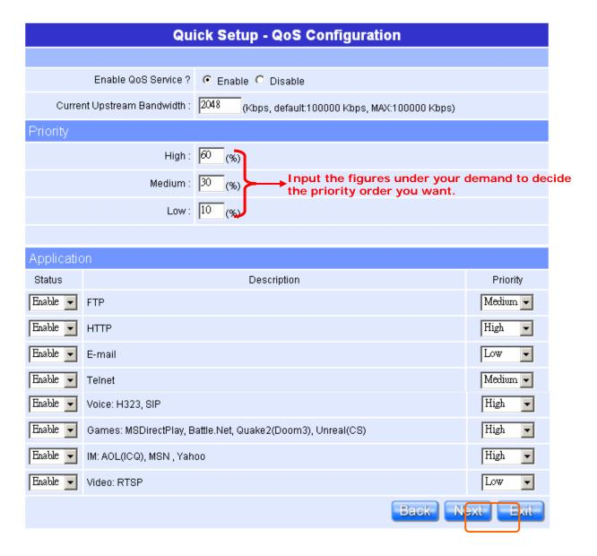
Make sure your connecting bandwidth with ISP and set the Priority percentage. Once setting the QoS service, the transmitting performance will be affected, so please ensure your connecting setting before doing this setup.
