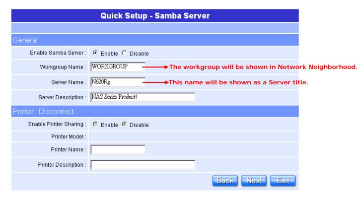
To set Samba Server by entering the information for group setting and printer, then click on "Next" button to connect to next setup after confirming. The name of printer in "Printer Server" and "Samba Server" can't be the same.
