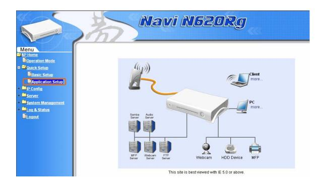
Notice: The Router Basic Setup should be done before setting the Application Setup.
