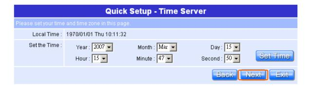
Select your time from the "Set the Time" drop-down list, there is no real time clock inside the router, the system date and time are maintained by external network time server.
