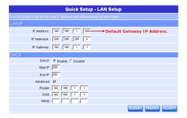
Please don't change the default LAN IP settings at this point until you have completed the rest of the configurations and confirm that your Internet connection is working.
