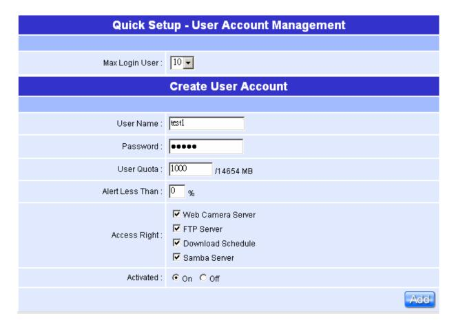
Set each user's right and space arrangement, then click on "**Add**" button for saving user's setting, and click on "**Next**" button after finishing.
