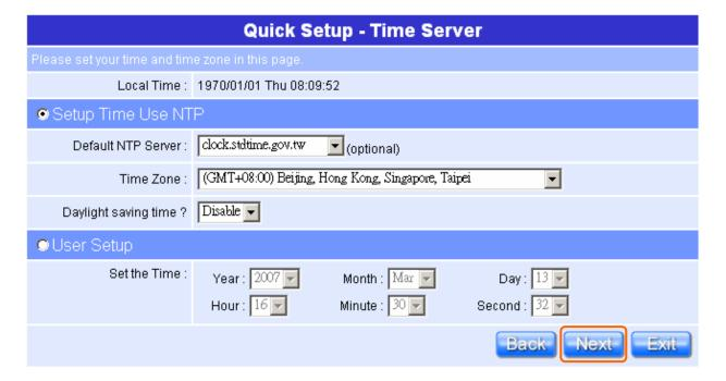
Select your time zone from the "Time Zone" drop-down list, there is no real time clock inside the router, the system date and time are maintained by external network time server.
