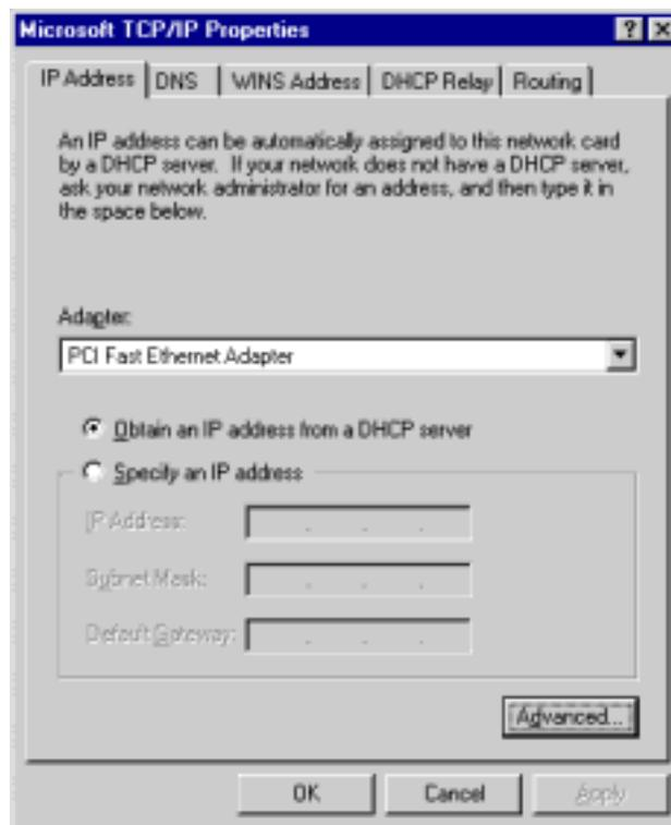
**Figure 68: Windows NT4.0 - IP Address**
