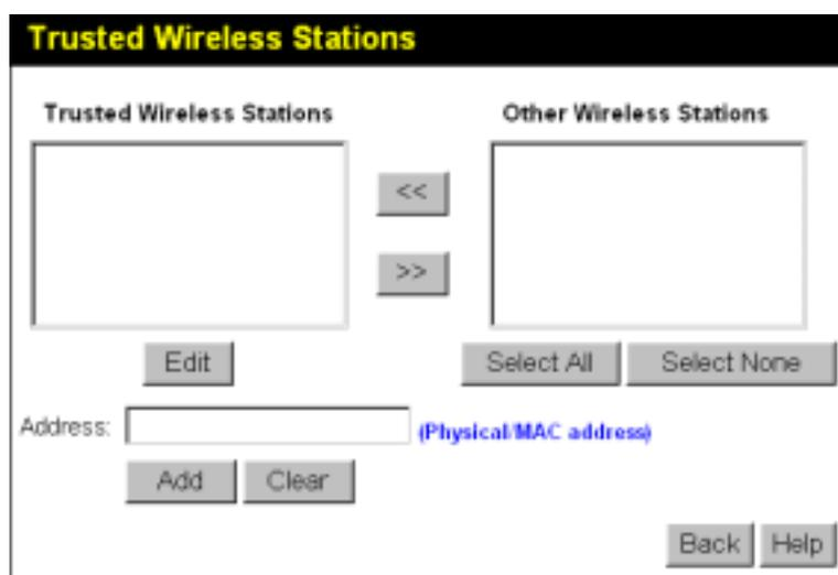
Figure 10: Trusted Wireless Stations
