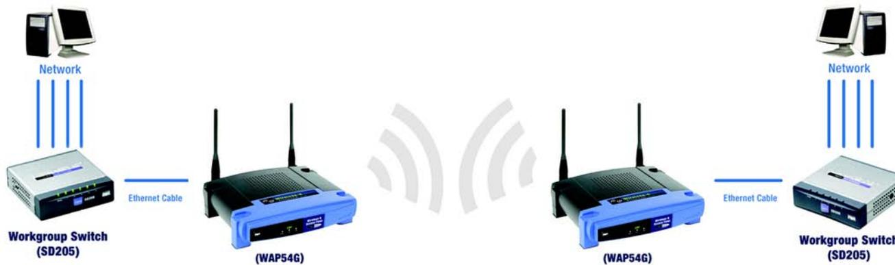
Figure 7-7: Wireless Bridge Diagram
