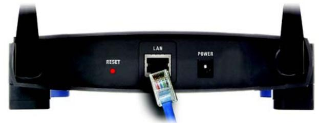
Figure 4-1: Connect the Ethernet Network Cable
