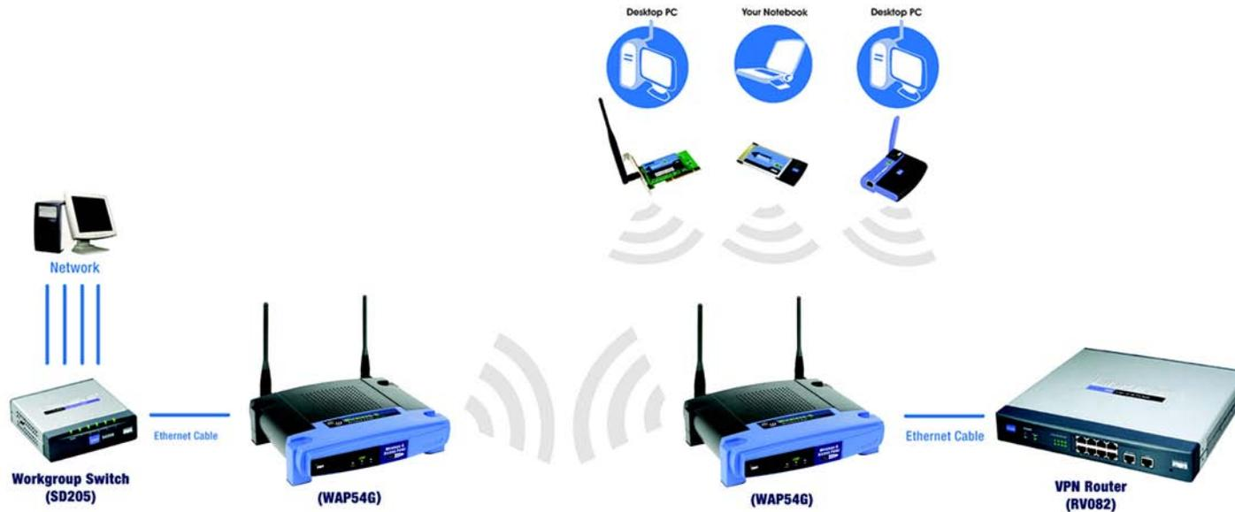
Figure 7-6: Wireless Repeater Diagram
