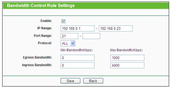
Figure 4-76 Bandwidth Control Rule Settings
