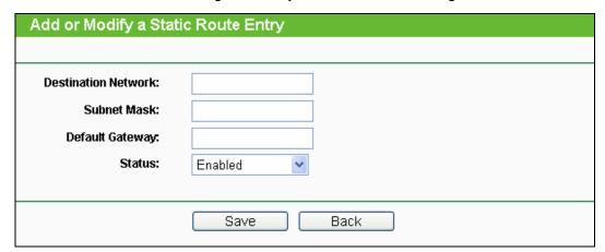
Figure 5-65 Add or Modify a Static Route Entry
