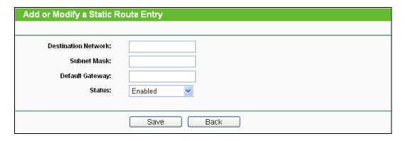
Figure 4-71 Add or Modify a Static Route Entry
