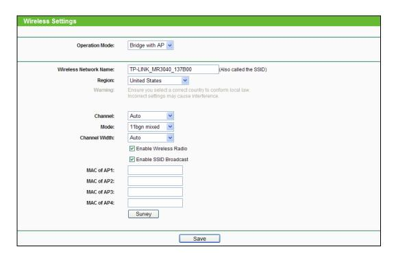
Figure 6-12 Wireless Settings in Bridge with AP mode
