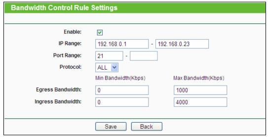
Figure 5-70 Bandwidth Control Rule Settings
