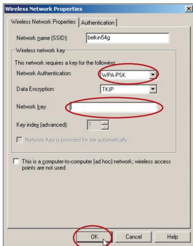
**Important:** WPA-PSK is a mixture of numbers and letters from A–Z and 0–9. For WPA-PSK you can enter 8 to 63 keys. This Network key needs to match the key you assign to your Wireless Router or Access Point.
