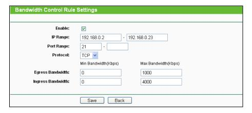
Figure 4-98 Bandwidth Control Rule Settings
