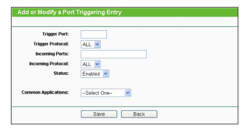
Figure 4-65 Add or Modify a Triggering Entry
