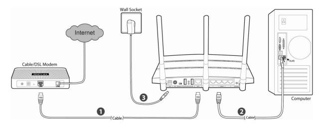
Figure 2-1 Hardware Installation
