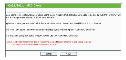
Figure 3-8 Quick Setup – MAC Clone
