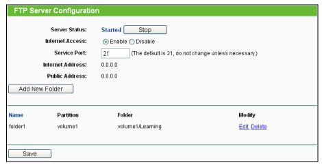
Figure 4-51 FTP Server Configuration
