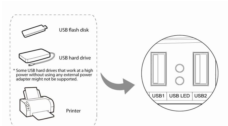
Figure 2-2 USB Installation
