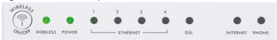
None of the LEDs are on if the ZyXEL Device is not receiving power.
