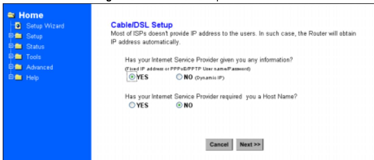
Figure 3-5 Cable/DSL Setup Menu with “No” Option Screen
