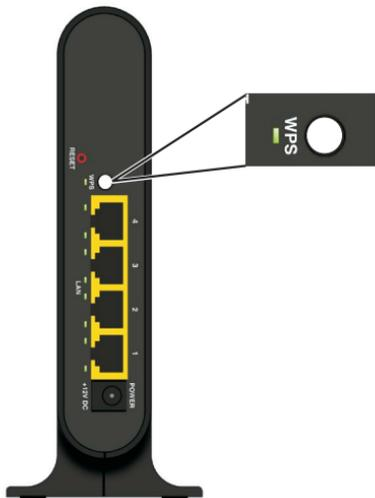
4. After the VAP establishes a wireless connection with your set-top box, the Wireless link LED lights:
