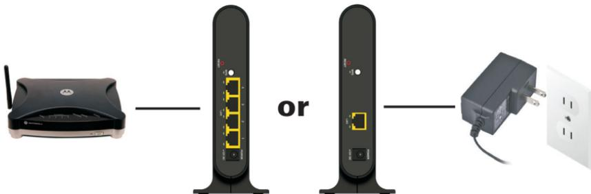
2. Connect the power adapter to the VAP and plug the adapter into a wall outlet. You'll see the power LED on the unit's front panel light green, indicating the unit is powered:
