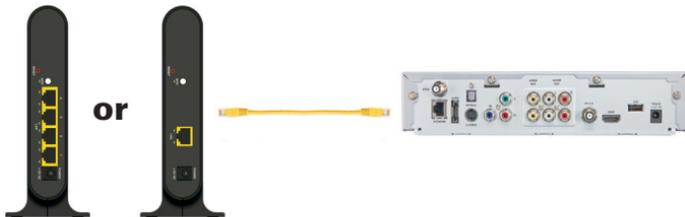
2. Connect the power adapter to the VAP and plug the adapter into a wall outlet. You'll see the power LED on the unit's front panel light green, indicating the unit is powered:
