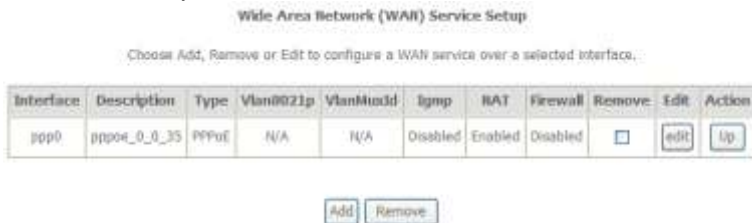
Figure 33 Completing the settings of PPPoE WAN service
