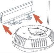
9. If the access point is not properly secured, press the release button on top of the bracket to unlock the access point. Realign the access point, making sure the cable is still connected, and push in on the access point until it clicks securely into place.
