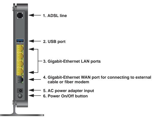
Figure 3. Back panel port connections
