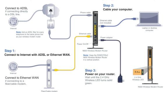
The installation guide that came in the box has a cabling diagram on the second page.
