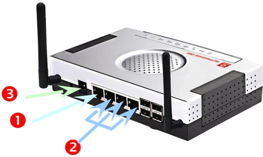
1. Connect an Ethernet cable from the cable/ADSL modem to the WAN port of the NetPassage 28G.
