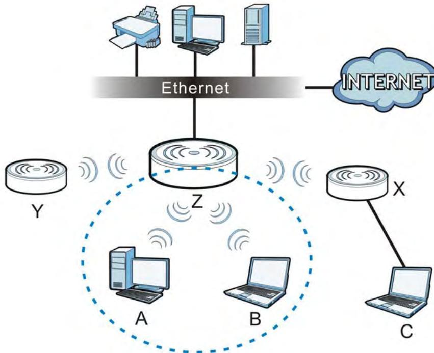
On the NWA in Root AP mode, you can have multiple SSIDs active for regular wireless connections and one SSID for the connection with a repeater (universal repeater SSID). Wireless clients can use either SSID to associate with the NWA in Root AP mode. A repeater must use the universal repeater SSID to connect to the NWA in Root AP mode.
