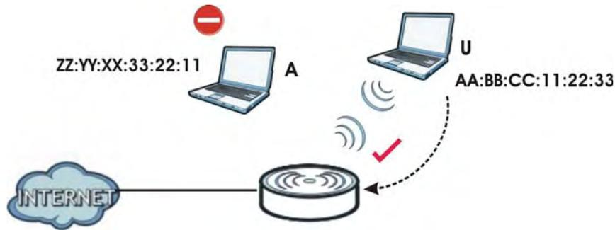
In the figure above, wireless client **U** is able to connect to the Internet because its MAC address is in the allowed association list specified in the NWA. The MAC address of client **A** is either denied association or is not in the list of allowed wireless clients specified in the NWA.
