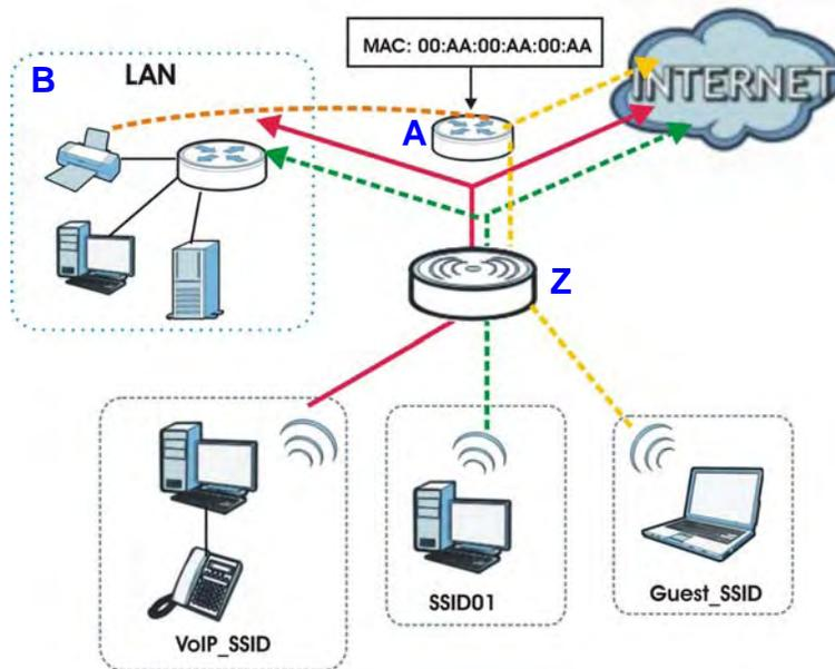
The standard network (**SSID01**) has access to all resources. The VoIP network (**VoIP\_SSID**) has access to all resources and a high QoS priority. The guest network (**Guest\_SSID**) has access to the Internet and the network printer only, and a low QoS priority.
