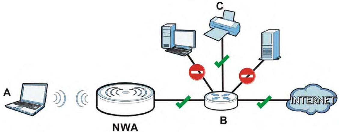
MAC addresses that are not listed in the layer-2 isolation table are blocked from communicating with the NWA's wireless clients except for broadcast packets. Layer-2 isolation does not check the traffic between wireless clients that are associated with the same AP. Intra-BSS Traffic allows wireless clients associated with the same AP to communicate with each other.
