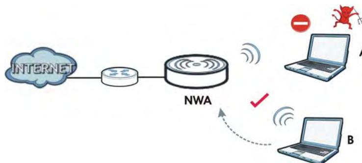
In the figure above, the NWA checks the identity of devices before giving them access to the network. In this scenario, Computer **A** is denied access to the network, while Computer **B** is granted connectivity.
