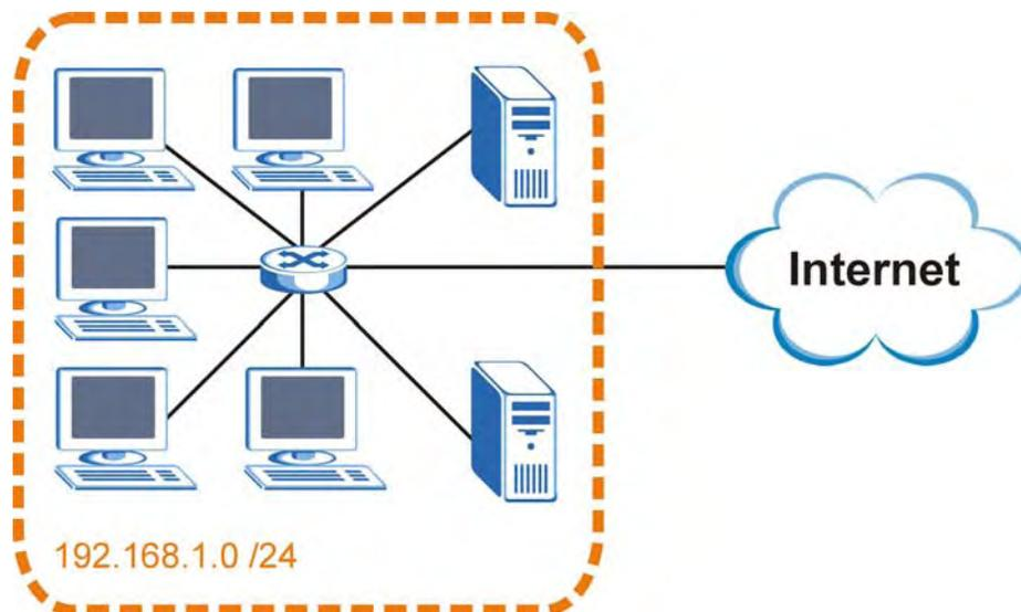
You can “borrow” one of the host ID bits to divide the network 192.168.1.0 into two separate sub-networks. The subnet mask is now 25 bits (255.255.255.128 or /25).
