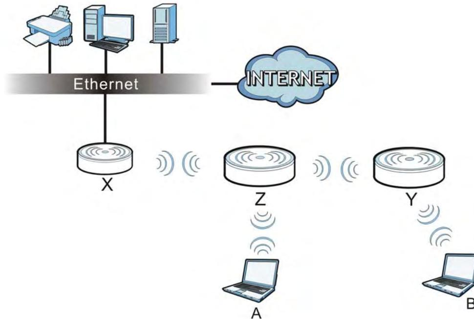
When the NWA is in Repeater mode, universal repeater security between the NWA and other repeater is independent of the security between the wireless clients and the AP or repeater. If you do not enable universal repeater security, traffic between APs is not encrypted. When universal repeater security is enabled, both APs and repeaters must use the same pre-shared key. See [Section 6.6 on page 76](#) for more details.
