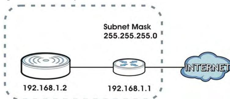
The figure above illustrates one possible setup of your NWA. The gateway IPv4 address is 192.168.1.1 and the IPv4 address of the NWA is 192.168.1.2 (default). The gateway and the device must belong in the same subnet mask to be able to communicate with each other.
