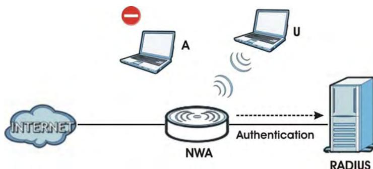
In the figure above, wireless clients **A** and **B** are trying to access the Internet via the NWA. The NWA in turn queries the RADIUS server if the identity of clients **A** and **U** are allowed access to the Internet. In this scenario, only client **U**'s identity is verified by the RADIUS server and allowed access to the Internet.
