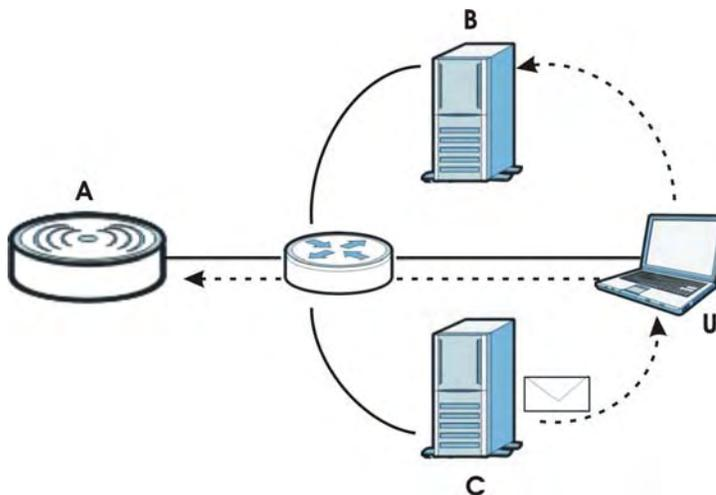
The figure above illustrates three ways to access logs. The user (**U**) can access logs directly from the NWA (**A**) via the Web configurator. Logs can also be located in an external log server (**B**). An email server (**C**) can also send harvested logs to the user's email account.
