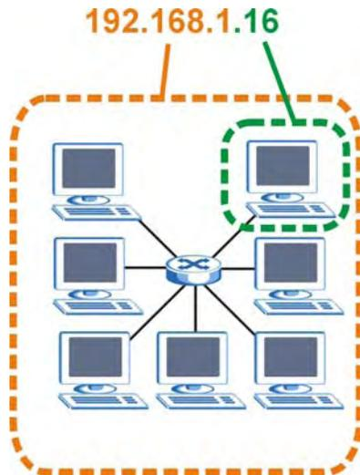
How much of the IP address is the network number and how much is the host ID varies according to the subnet mask.
