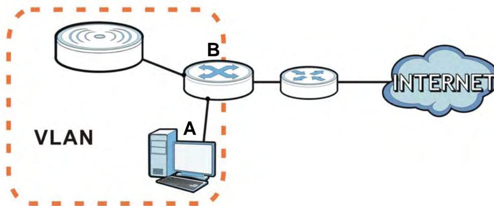
In the figure above, to access and manage the NWA from computer **A**, the NWA and switch **B**'s ports to which computer **A** and the NWA are connected should be in the same VLAN.
